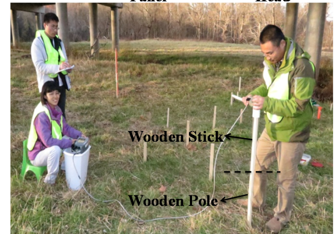
Magnetometer Setup and Operation
