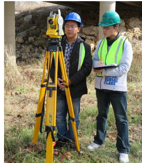
Total Station and Prism for Positioning
