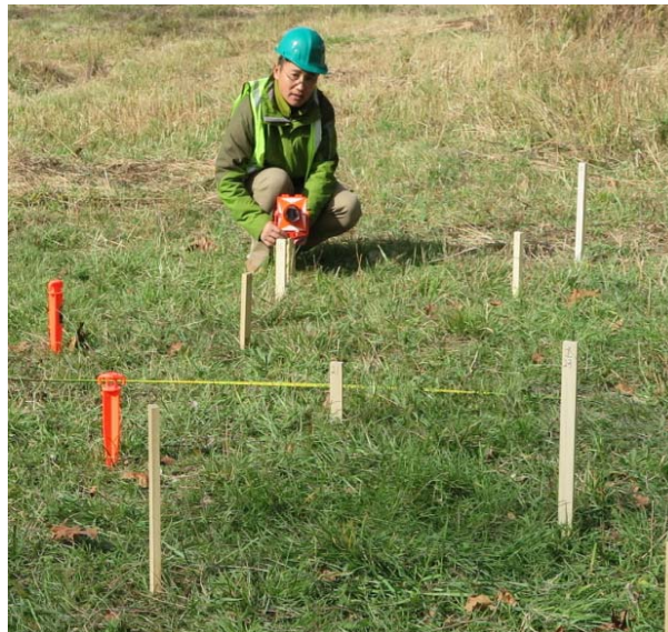
Total Station and Prism for Positioning
